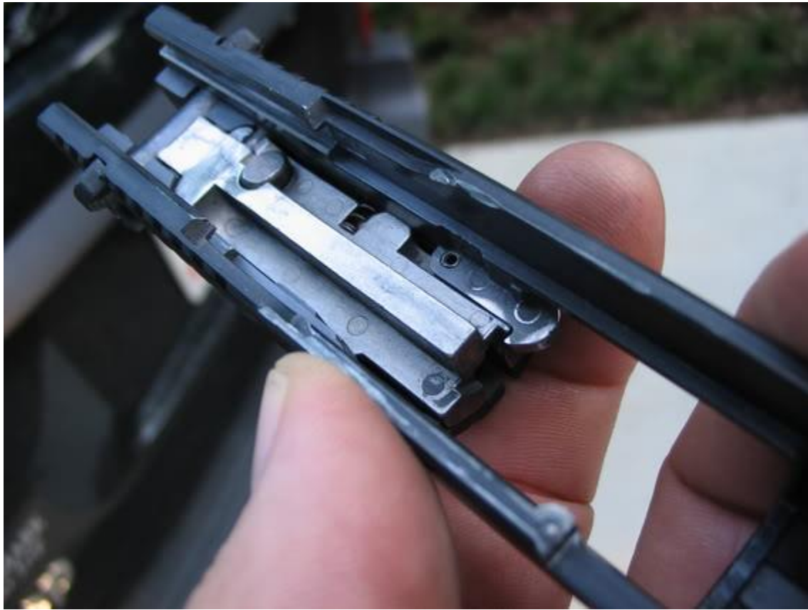
Extractor pin reinstalled and seated flush.
